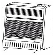
Figure 7 - Removing Lower Front Panel Of Heater
